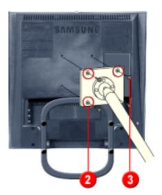
Align the four bolt holes (1) on the monitor base with the holes (2) on the VESA base and then fasten the base with the four bolts (3) supplied.
